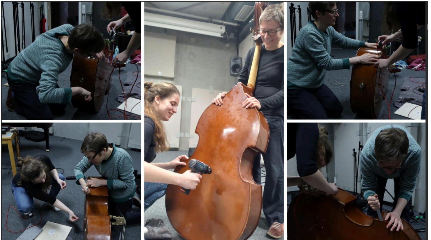
Figure 2: Opening the doublebass to insert the transducers with the help of the violin maker Annegret Mayer-Lindenberg
