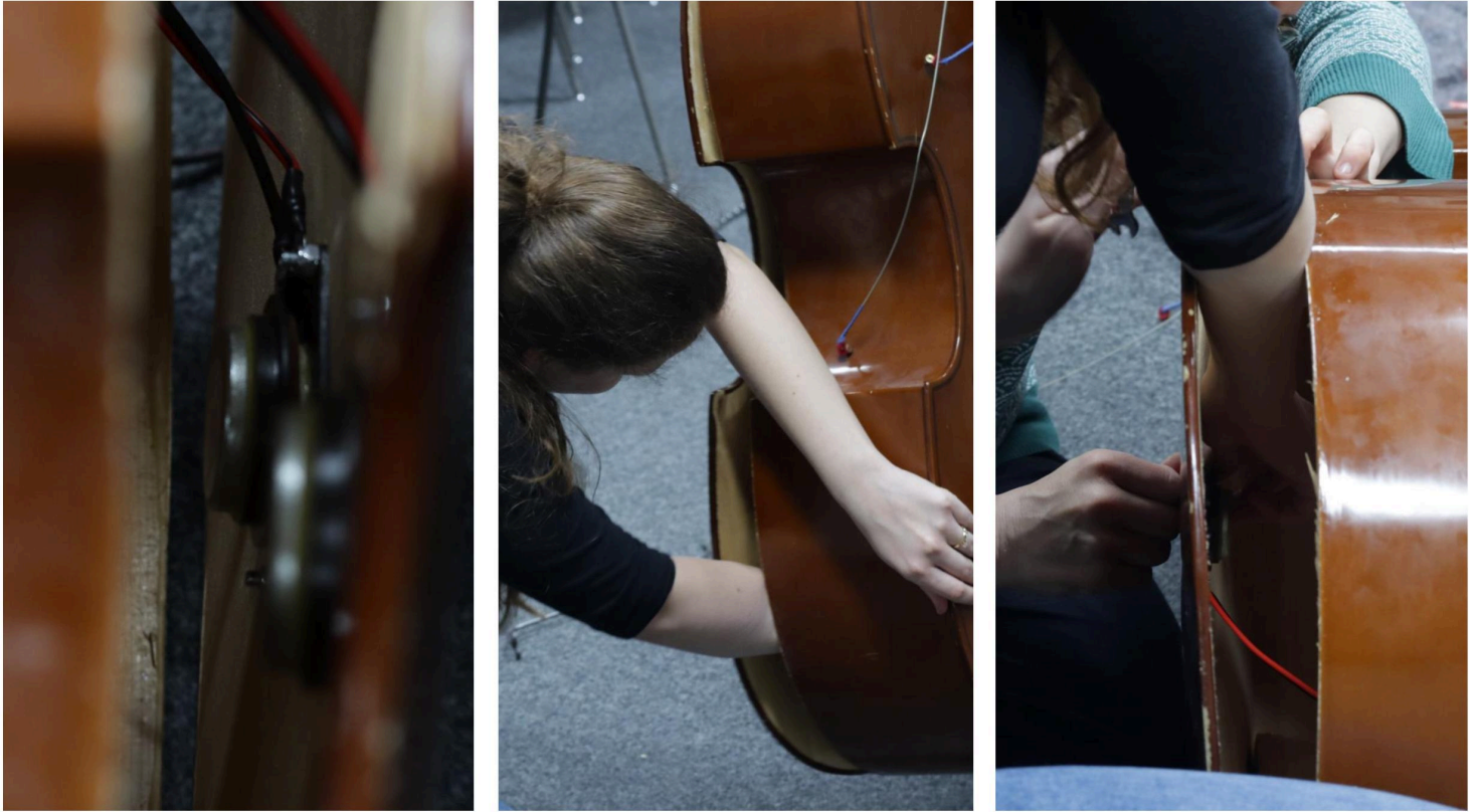
Figure 3: Setting the transducers into the bass
